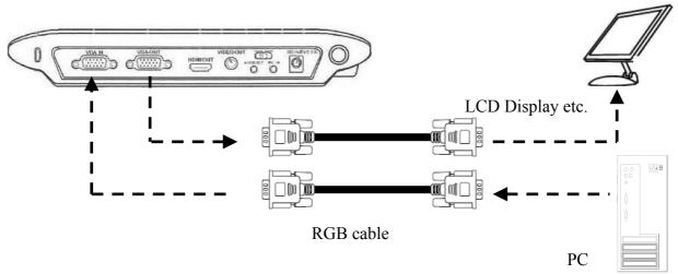
To display the PC image, press the PC button on main unit, and switch the document camera to PC mode.
