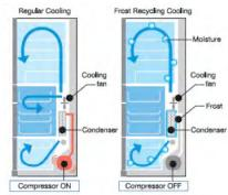
With Regular Cooling systems frost formed on the evaporator simply melts and is discarded.
