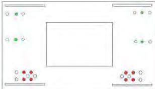
Using parts 4, mount into the holes marked Red Using parts 6, mount into the holes marked Green
